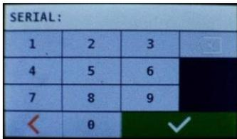
Enter the unit serial number located on the lower left side of the oven, be sure to include the three preceding digits at the end. Press the green check to continue to the home screen.
